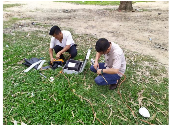
Resistivity survey for groundwater exploration at Dimapur Stadium
