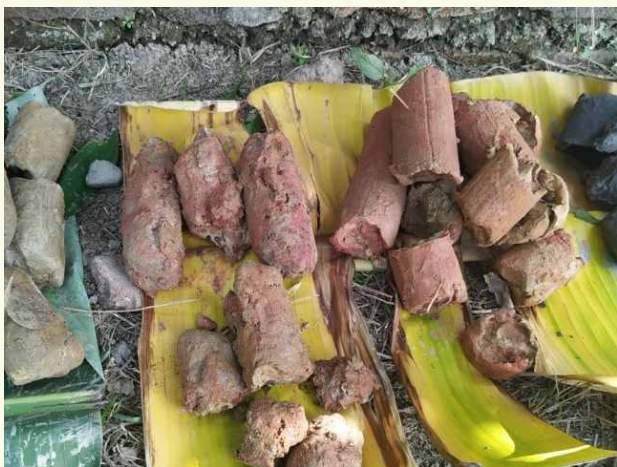
Core sample collection for sub-surface strata correlation. Loc: City College of Commerce
