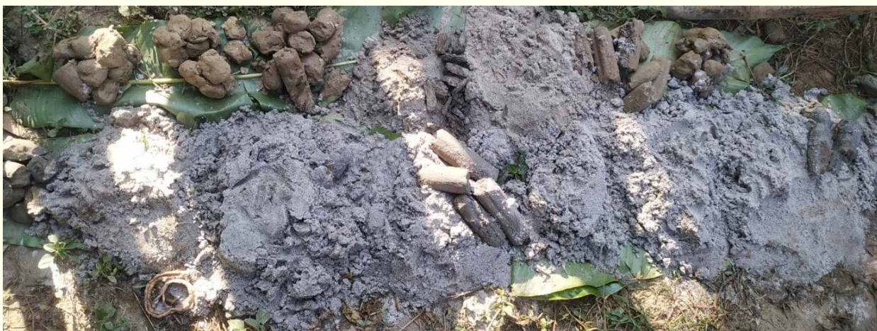
Core sample collection for sub-surface strata correlation. Loc: Kushiabil
