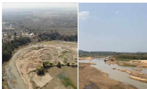
Pic: Unregulated sand mining altering river course and eroding banks causing flooding in low lying areas.
